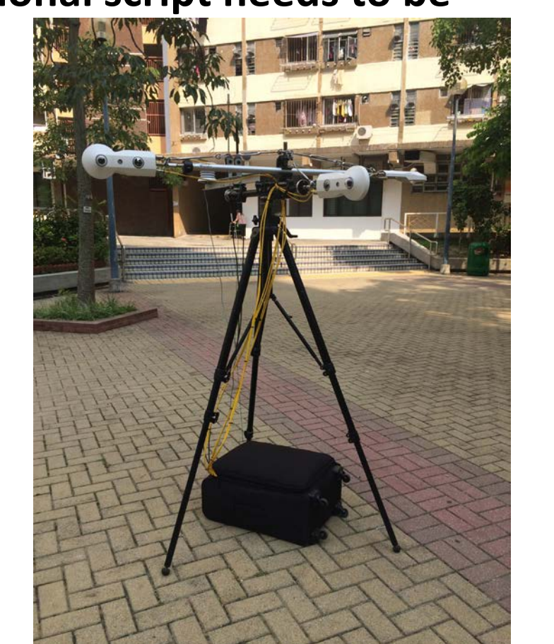
Figure 4.0: CNR 4 and globe thermometer setup
